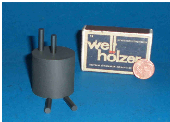
Graphitform, kleinformig Graphite mould, small format
